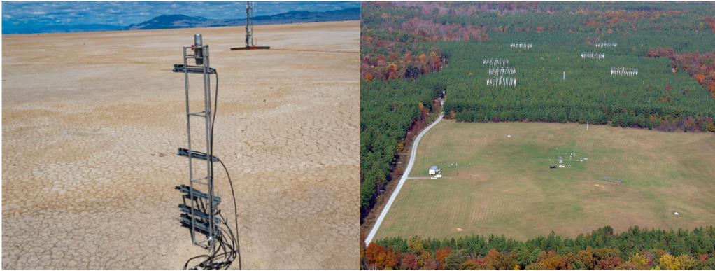
Figure 2. Left: The 1-m vertical array of nano-scale sensors at the SLTEST site. Right: The Duke Forest Grass Clearing site.
