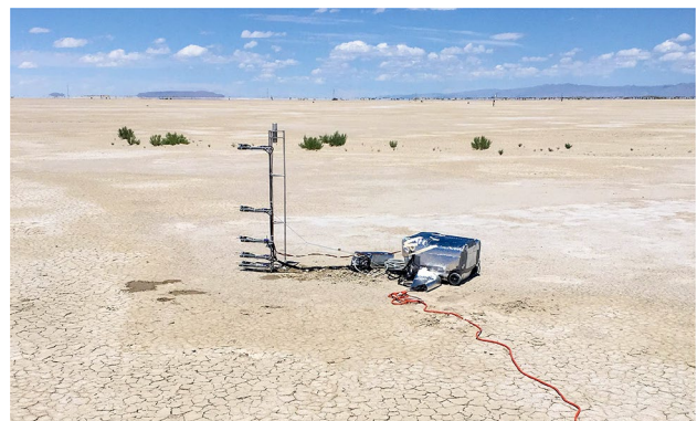
Fig. 6 Measurement tower of 1\text{ m} height, with acquisition systems placed downwind and covered with reflective material
